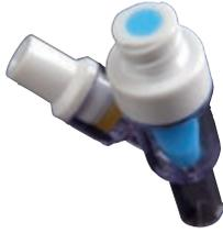
The needleless access connector Y-site with integrated check valve was made with Makrolon® Rx1805 polycarbonate resin. The check valve features increased resistance to chemical attack from intravenous fluid products, such as lipid emulsions, and “true swabability,” meaning the valves can be readily disinfected and reactivated.
