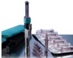
This needleless injection system can be used for many different liquid medication that have to be administered subcutaneously. The chosen Makrolon® grade has the advantage to withstand gamma irradiation sterilization without yellowing and pressures up to 30 MPa during injection.
